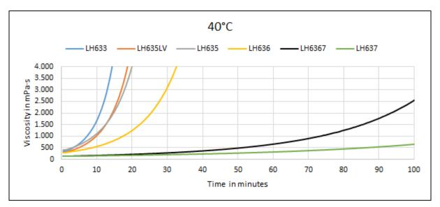
Measuring conditions: Viscometer, cone-plate configuration, diameter 50 mm, gap 0.1 mm
