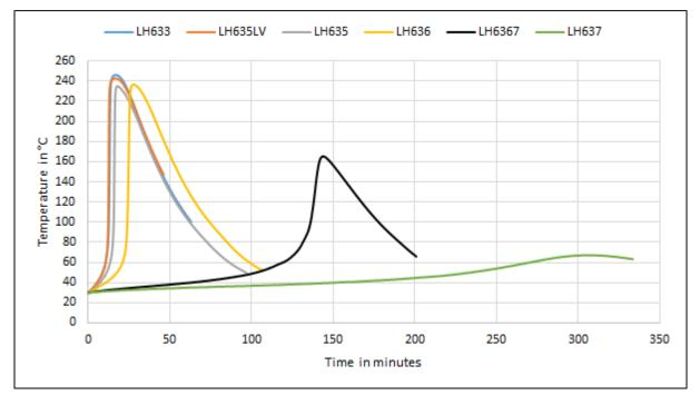
Measuring conditions: measured 100g in a paper cup isolated in a water bath at 30°C
