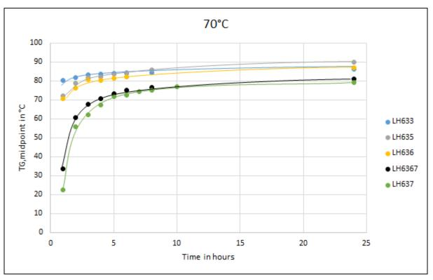
Measuring conditions: DSC-measuring heat rate: 20°C/min, sample mass 10-20 mg
