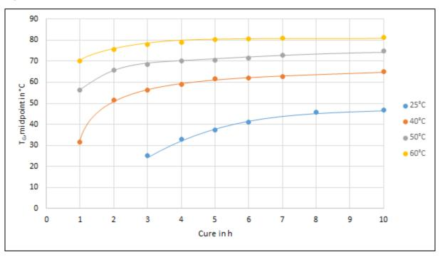
Measuring conditions: DSC-measuring heat rate: 20°C/min, sample mass 10-20 mg
