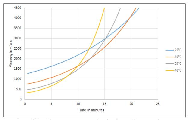
**Measuring conditions:** Viscometer, cone-plate configuration, diameter 50 mm, gap 0.1 mm
