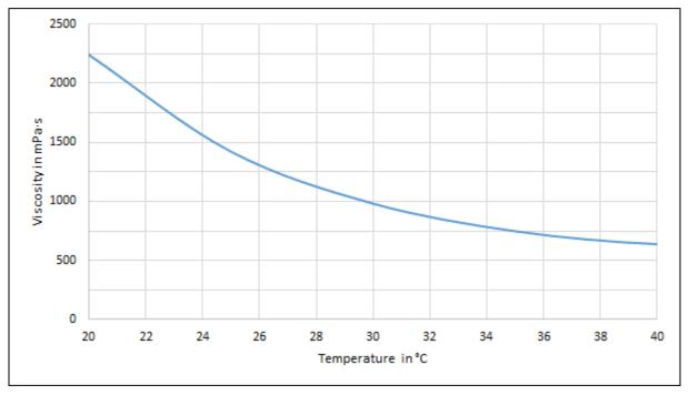
Measuring conditions: Viscometer, cone-plate configuration, diameter 50 mm, gap 0.1 mm
